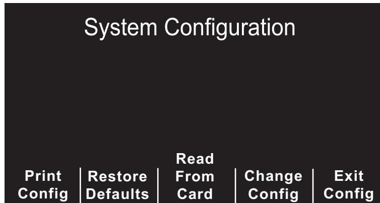
This menu provides the following five (5) softkey options: **Print Config**, **Restore Defaults**, **Read From Card**, **Change Config**, and **Exit Config**.
