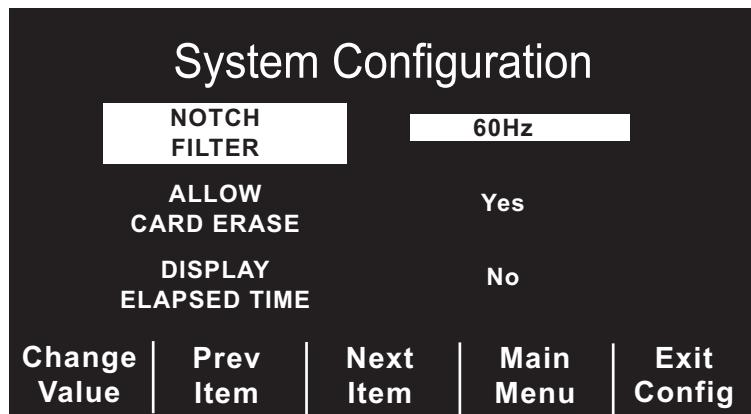
The name of each configurable feature is displayed in the left column of the option menu and that feature's current setting is shown in the right column.
