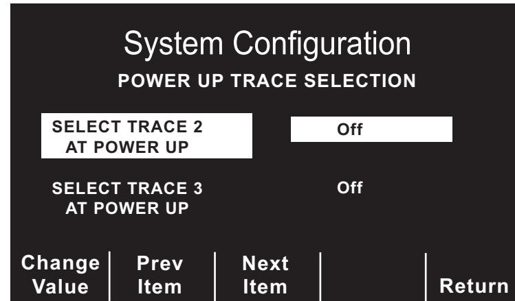
Press the **Change Value** softkey to scroll through the available parameters for each Trace selection.
