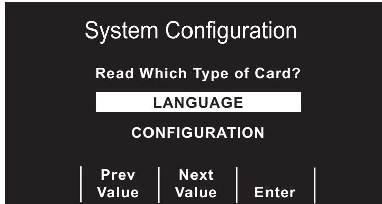
To move the highlighted area from LANGUAGE to CONFIGURATION and vice versa, press the **Prev Item** and **Next Item** softkeys. Press the **Enter** softkey to begin reading and storing the language settings or configuration settings from the user installed memory card.
