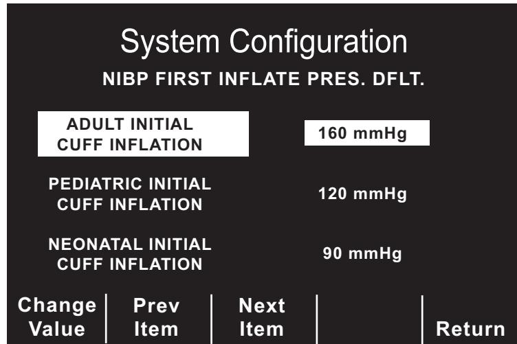
Pressing the **Change Value** softkey will scroll through the available inflation pressures for the highlighted parameter.
