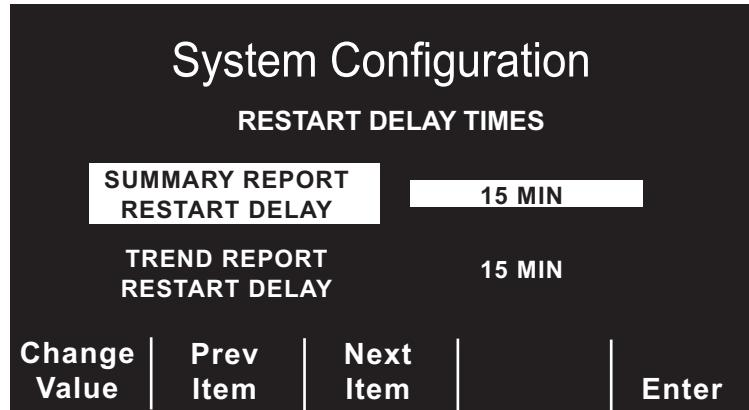
Pressing the **Change Value** softkey will scroll the highlight through the available delay times.
