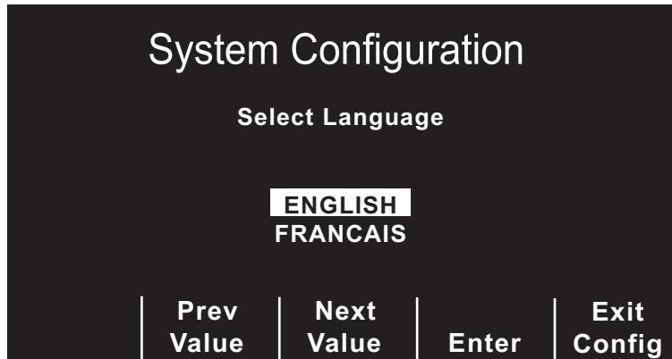
The first configurable option displayed after entering the correct pass code is the Select Language option. Press the **Prev Value** and **Next Value** softkeys to move the highlight from one language to the other.
